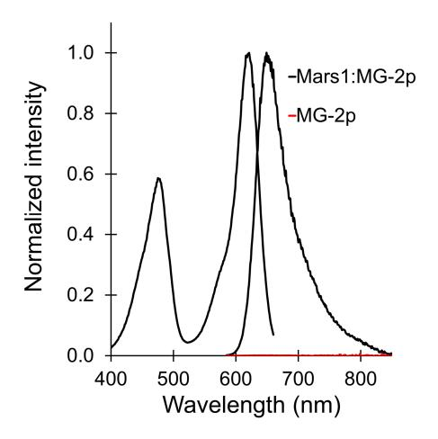
Supplemental Figure 2. Excitation and emission spectra of Mars1:MG-2p and emission spectrum of free MG-2p in PBS, pH 7.4. Mars1Cy:MG-2p and corresponding fluoromodules formed with MG-ester, a membrane-permeant derivative of MG-2p, are highly similar and omitted for clarity. Excitation peaks of the fluoromodule occur at 478 and 621 nm, enabling use with 488 and 633 nm laser lines. The wavelength of maximum emission lies at 649 nm.
